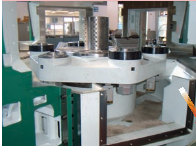
Hirth crown gear for highly accurate indexing of the satellite table
